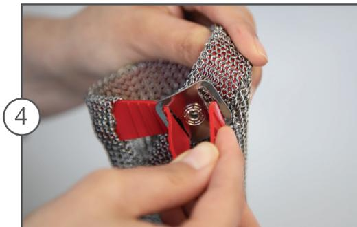
Slide the wristband back into place on the clip and put on the glove
