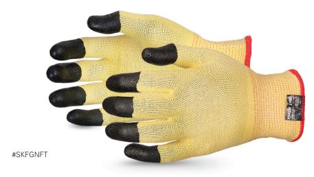
This cut-resistant 13-gauge knit is highly dexterous, yet provides stellar cut protection. Composite blend of Kevlar® wrapped around composite filament fiber provides ASTM level-4 cut protection, withstanding 1650 grams of cut force during testing.
