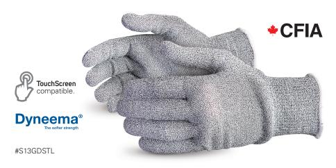
Fine-gauge gloves are knit with a composite yarn that offers ANSI level A5 cut protection - remarkable for a 13-gauge glove. That's 2620 grams of cut resistance thanks to a blend of Dyneema® and stainless steel, and because they are also treated with AlphaSan® - an antimicrobial agent — they are ideal for the food and beverage industry.
