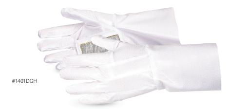
The base fabric of our gloves is a 1 mil polyurethane film laminated to a knitted nylon backing. The material has a soft feel and inherent lint free properties. We sew this material using an UltraSonic sewing process, bonding edges and seams. Edges are sealed with no stitch, preventing penetration of fluids.
