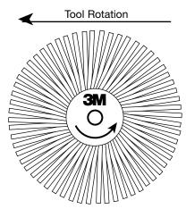
Refer to directional arrow on disc for proper loading on tool.
