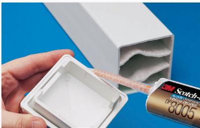
3 With no surface preparation, 3M™ Scotch-Weld™ Structural Plastic Adhesive DP8005 bonds end caps on Low Surface Energy plastic fence posts. Handling strength in 2-3 hours.
