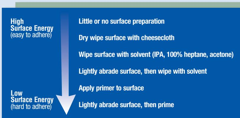
Graphic shows surface preparation methods which may be required to maximize bond strength.
