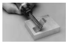
Flat surface 2" x 2 <sup>1</sup>/<sub>4</sub>" peened to 12 Almen "A" intensity with a 9/16" x 1 <sup>1</sup>/<sub>4</sub>" flap.
