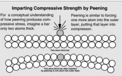
The inner layer is in tension. Since both layers are bound together, differences in elongation cause the bar to bend. Realistically, both layers are several mils thick and the bar is too thick too bend. The outer layer remains in compression; the layer below remains in tension.
