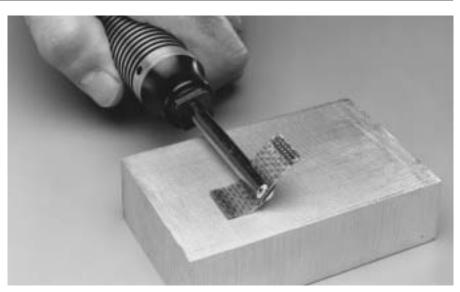
Peen surface with a circular motion. Tool must be pre-set to a constant torque.
