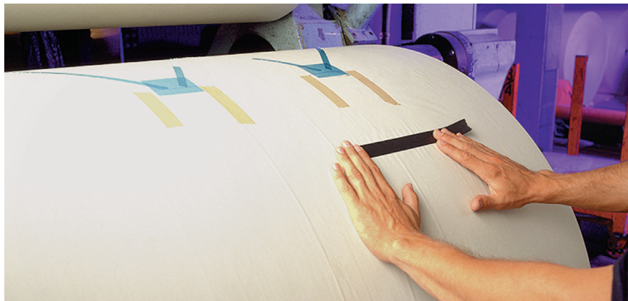
To mark a roll with opaque black crepe tape to signal a knife cut during a splicing operation, you can select either the 5.6 mil thick 3M™ Crepe Masking Tape 2510 or the 7.0 mil thick 3M™ Photographic Light Blocking Tape 235. With conformable backing and rubber adhesive, both tapes hold securely at full operating speeds.
