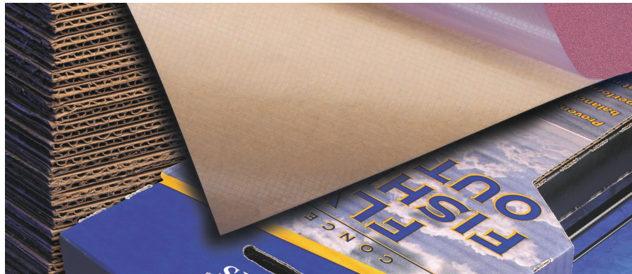
Designed specifically for flexographic printing on corrugated board, 3M™ Thin Flexographic Mounting Tape 2205 is a 5-mil double-coated polyester film tape with cross-hatched adhesive. The cross hatching reduces air entrapment, saving time and improving print quality.
