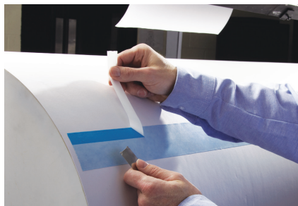
One simple splice with 3M™ Splittable Flying Splice Tape replaces complex patterns.
