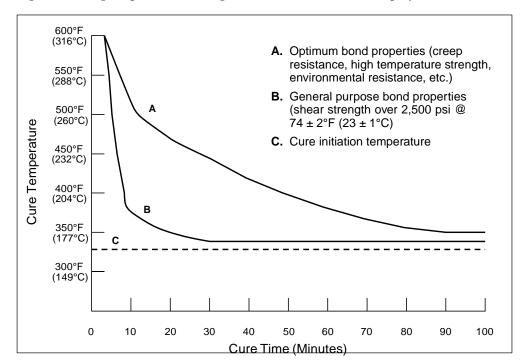
Figure 1 – Curing Temperature vs Curing Time for 3M<sup>™</sup> Scotch-Weld<sup>™</sup> Epoxy Adhesive EC-1386
