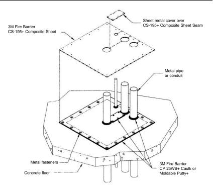
**C.** Penetration Firestop for Insulated Metal Pipe through a cement block or concrete wall. Refer to current UL Fire Resistance Directory for system numbers.
