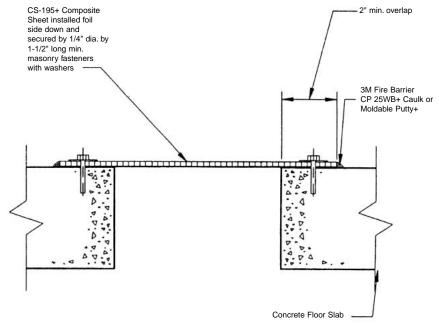
**B.** Penetration firestop for large openings with pipe using CS-195+ Composite Sheet. Refer to current UL Fire Resistance Directory for system numbers.
