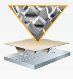
3M precision-shaped grain uses 3M microreplication technology to form sharp peaks that easily "slice" through metal – cutting cooler, faster and lasting longer than conventional abrasive grain. That means more consistent performance with fewer disc changes – so you can get more work done over the life of your disc.
