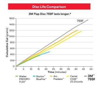
\* Results based on an automated test on mild steel using 4.5 inch flap discs with constant tool power until end of life, using grade 40+ or nearest equivalent.
