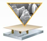
Conventional abrasive grain tends to "plow" through the metal, causing heat to build up in the workpiece and the abrasive — resulting in a slower, less consistent cut and shorter disc life.
