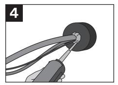
Fill all voids and interstices of cables with 3M™ Fire Barrier Rated Foam FIP 1-Step, full depth of the plug.
