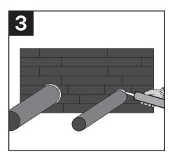
Install 3M™ Fire Barrier Rated Foam FIP 1-Step between the blocks/planks and the periphery of the opening and between blocks/planks and penetrants. Foam to be installed full depth of the blocks/planks. Check for any openings between blocks/planks, framing and penetrating items. Fill any visible openings with the required depth of foam.
