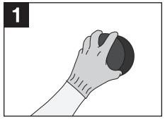
Install 3M<sup>™</sup> Fire Barrier Plug within the opening, flush with top surface of floor or both sides of wall. To fit smaller openings, plugs may be compressed to size or a wedge may be cut from plug to reduce size.
