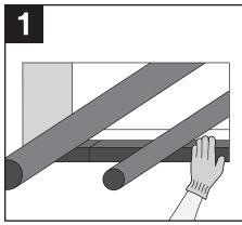
Install 3M™ Fire Barrier Blocks/Planks with the 5 in. (130mm) dimension projecting through the floor or wall and centered within the opening. Blocks/planks should be installed so the integrated grid is not in contact with the substrate or in a grid-to-grid manner.
