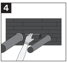
To remove the blocks/planks, gently pull them out and place on a clean surface. After penetrants are routed through or removed from the opening, replace the blocks/planks, making sure that they are firmly packed and fully filling the opening. Install foam in any voids as required.
