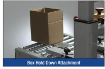
Holds RSCs on the optional infeed conveyor to free the operator's hands for case filling.
