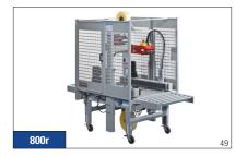
3M-Matic™ Case Sealer 800r is a semi-automatic random case sealer automatically adjusts for case height and width. Top and bottom seal at rates up to 20 cases per minute, using tape widths from 36mm to 48mm wide.
