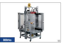
3M-Matic™ Case Sealer 800rks is a random king size case sealer that automatically adjusts for case height and width and is capable of sealing up to 10 cases per minute, using tape widths from 48mm to 72mm wide.
