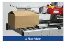
For increased productivity, easily attached flap folder assists operator in folding the minor (front) and two major (side) flaps of RSCs before taping.
