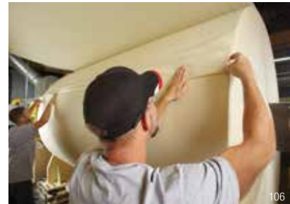
For finished mill overlap splicing, 3M™ Repulpable Permanent Tape provides high shear strength without adhesive oozing or bleed through.
