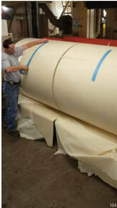
High tack 3M™ Temporary Single Coated Repulpable Tapes are available in white, blue, and kraft for dependable core starting, roll closing and butt splicing.
