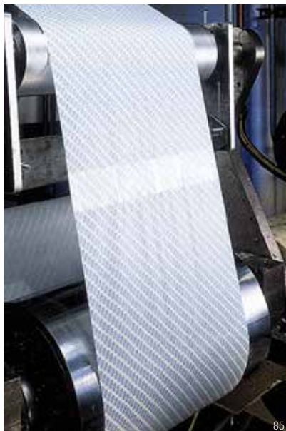
For butt splices on many low surface energy materials such as polyethylene, 3M™ Super Bond Film Tape 396 provides the thin caliper tensile strength of polyester, and high immediate holding strength of rubber adhesive.
