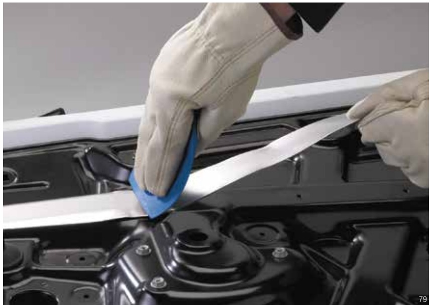
Applied with a 3M™ Plastic Squeegee PA-1 Wiper to the inside of a car door, 3M™ Damping Foil 2552 effectively damps noise and vibration with as little as 10% surface coverage. Optimized acrylic on a dead soft aluminum constraining layer converts vibrational energy to negligible heat that readily dissipates.
