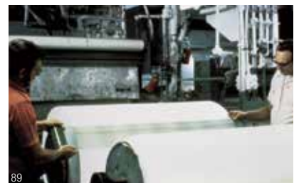
With thin caliper, high tensile strength polyester backing and the excellent shear strength of silicone adhesive, 3M™ Polyester Tape 8402 works well for butt splicing silicone-treated papers.
