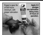
• Lubricate wick system through the angle gear oil fitting with 2-3 plunges for every 24 hours of use, to achieve maximum gear life. Prime pump to insure good oil flow.
